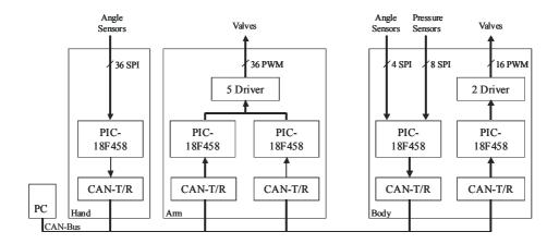
**Fig. 9.** The above shows a schematic plan of the connections of the hand (left) and shoulderarm (right) electronic devices. The hand consists of two boards, one for sensor inputs and one for valve outputs, which communicate via CAN. The shoulder-arm electronic, in brief 'body', is configured as one printed board and located in the robot's base
