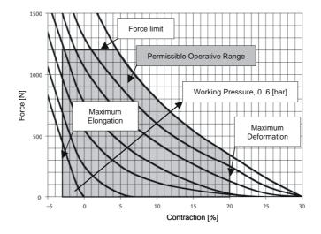
**Fig. 8.** This diagram shows the relationship of the possible produced tractive force in Newton to lift up something to the affordable contraction rate expressed in percentages of the basis length by a given working air pressure in bar of the fluidic muscle MAS-20
