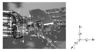
**Fig. 6.** *Left*: A photograph of ZAR's wrist joint with axes 1 points to a Bowden cable which connects the muscle actuator (fixed end) with a finger root joint inside the palm. 2 points to the tendon which drives the hand lift joint and 3 to the tendon attached to the tilt joint of the wrist. *Right*: The depiction of the corresponding Cartesian coordinate system of the wrist
