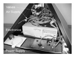
**Fig. 2.** The photograph above shows an inside view of the base which contains the power supply for 24 V and 5 V, the electronic devices for the shoulder and arm, the air tubes for supply and delivery directly connected to the valve cluster and the on-off valves for the shoulder and arm placed on a valve cluster.
