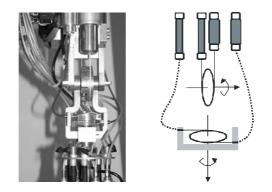
Fig. 5. *Left*: A photograph of the actual elbow joint is shown. *Right*: The redirection of the muscle-tendon systems and the displacement of the Bowden cables (dotted lines) are traced
