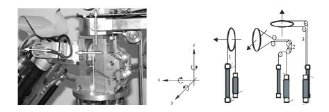
**Fig. 4.** *Left*: This is a photograph of the shoulder joint of ZAR3. The numbers 1,2 and 3 indicate the tendons of the x-, y- and z-axis of the joint. *Middle*: Shows the relation of the rotary directions to Cartesian space. *Right*: Clarification of the muscle-tendon systems and the redirections caused by the mechanical constraints and the acting pulley to drive the distal segments
