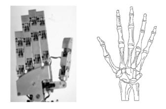
**Fig. 7.** *Left*: A photograph of the five-finger hand in home position. The dark spots between lighter surfaces are recesses to afford the bending of the phalanxes. *Right*: A view of the bones of a human hand is shown; the similarities are clearly visible
